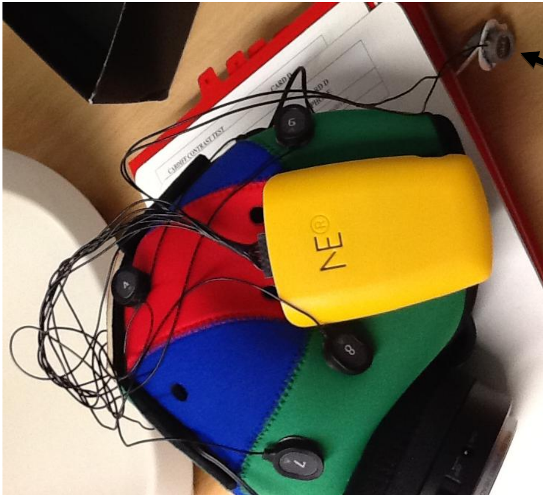
Fig. 4 Stick-on electrodes to DRL and CMS cables
